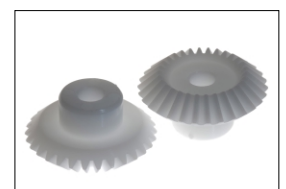
Pt No. 919D25. Nylon Bevel Gears 1:1. OD30.7mm ID 6mm. Module 1.0. 6g
