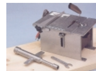
CIRCULAR SAW. Pt.No. 925D For use with 400DHD. 12-18v DC.Power 100watts. Blade height adjustment. guide for cutting angles.
