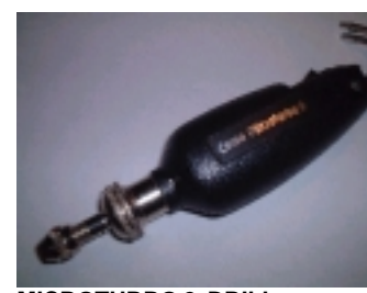
MICROTURBO 2. DRILL. Pt.No. 587D 6-18V, 14500 r.p.m., Torque 530g.cm, collet chuck. Shaft runs in precision ballrace.
