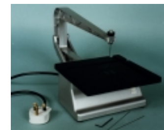
ELECTRIC FRETSAW. Pt.No. 933D 240v AC mains operation with built in heavy duty transformer. 5v 5 pole low voltage motor. Fully rotatable blade. Max cutting height 75mm, cutting stroke 5mm, cutting strokes per min. 1500. Throat depth 295mm, table dims. 197mm x 197mm.
